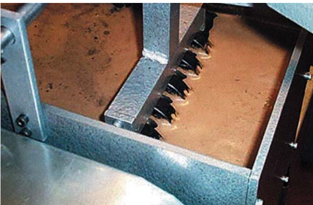
The various seal designs show a different level of performance in the contaminated environment of application.
